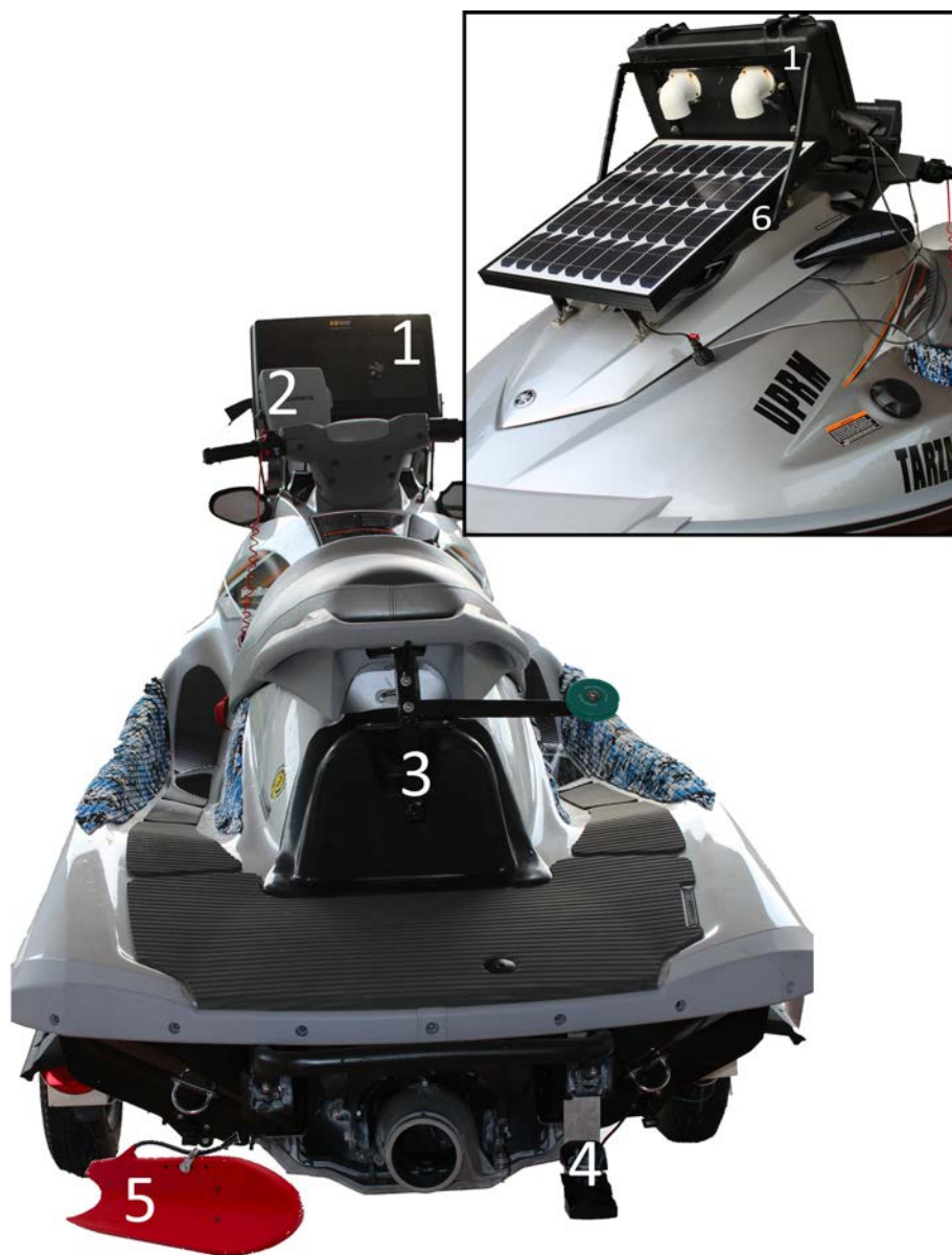
Figure 3.1: Personal watercraft instrumentation: (1) watertight laptop case; (2) Garmin GPS receiver; (3) side scan sonar tow stand; (4) single beam echo-sounder (SBES); (5) Starfish side scan sonar; (6) solar panel.
