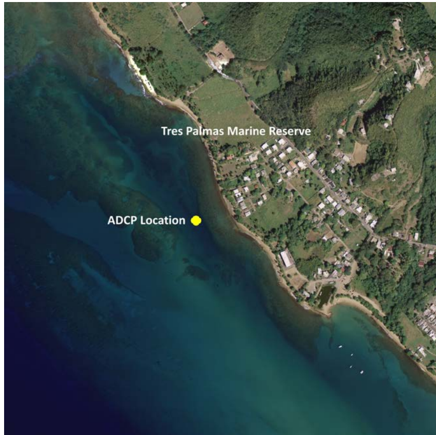
Figure 4.9: Location of the Acoustic Doppler Current Profiler (ADCP) deployed in the Tres Palmas Marine Reserve during the model validation period from January 11, 2013 through February 22, 2013.
