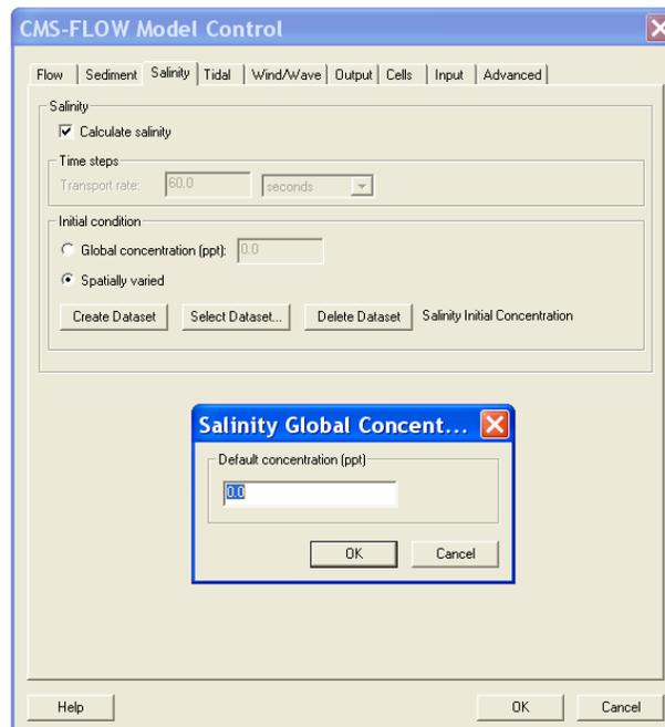
Figure 2-71. Setting up the salinity calculation and specifying spatially varied initial salinity.
