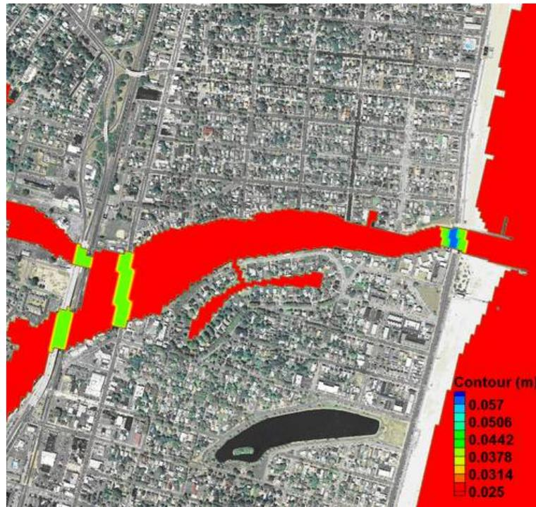
Figure 2-10. Manning's  $n$  contours after modifying the areas under all three bridges.
