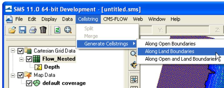
Figure 2-36. Automated Cellstring generation in SMS 11.0
