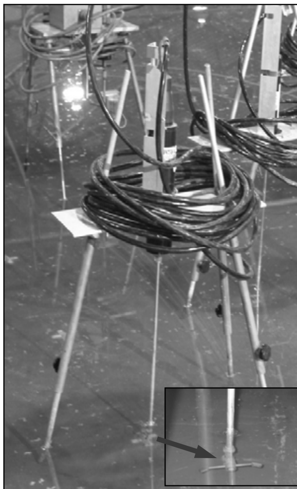
Figure 7. Acoustic Doppler Velocimeter
