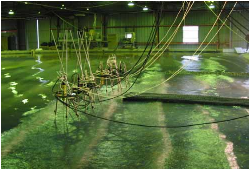
Figure 12. Current meters seaward of jetty
