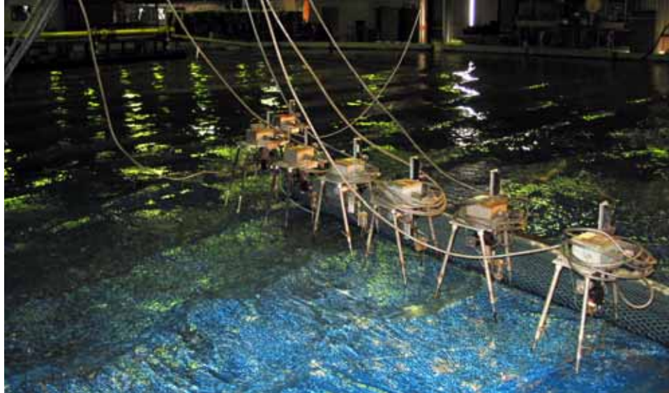
Figure 11. Wave gauges near jetty
