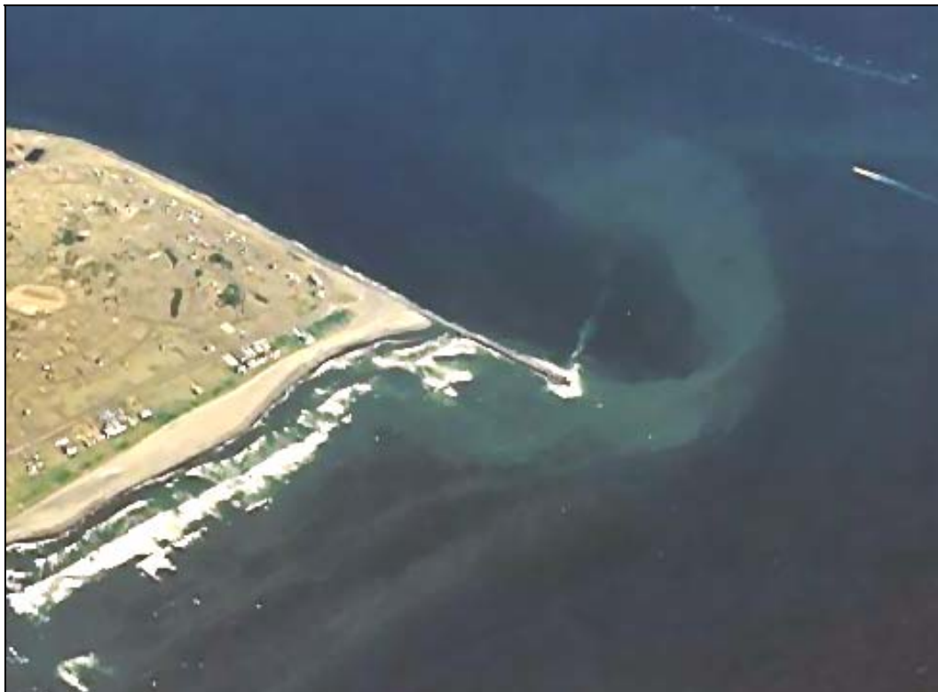
Fig. 1. Wave-generated longshore currents at Grays Harbor, WA, during flood tide
