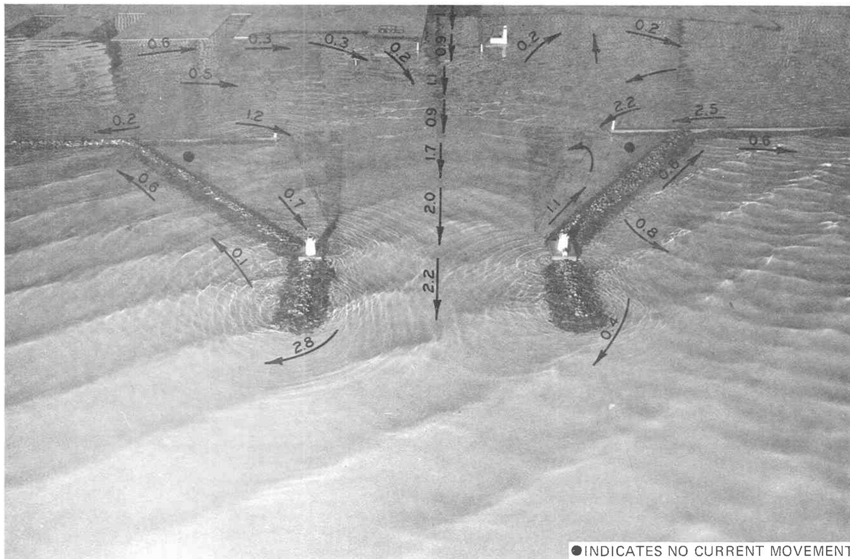
Photo 74. Typical wave patterns, current patterns, and current magnitudes (prototype feet per second) at the west entrance for Fair-Weather Plan 4D; 9-sec, 8.6-ft waves from 279 deg; +4.8 ft swl; river discharge 8,000 cfs
