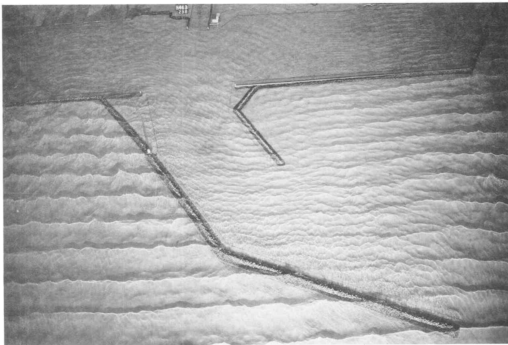
Photo 154. Typical wave patterns for Severe-Weather Plan 15; 10-sec, 13.7-ft waves from 326 deg; +4.8 ft swl; river discharge 800 cfs
