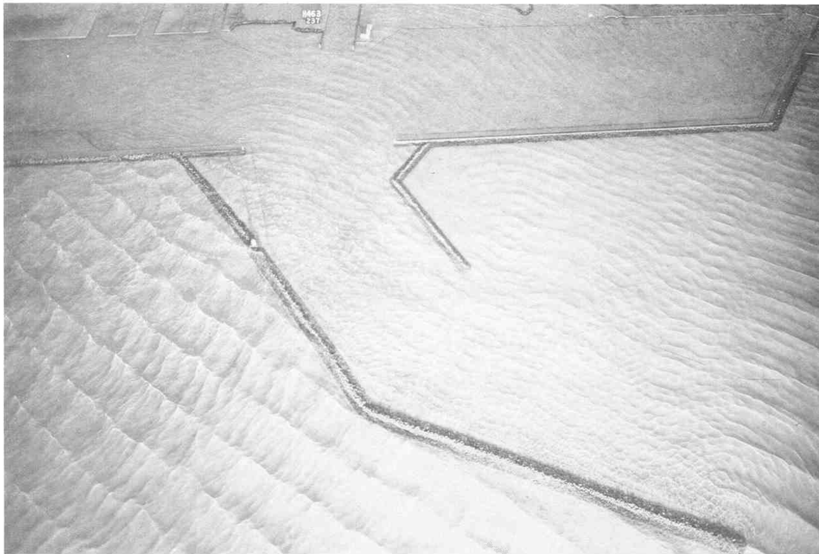
Photo 156. Typical wave patterns for Severe-Weather Plan 15; 9.5-sec, 12.2-ft waves from 17 deg; +4.8 ft swl; river discharge 800 cfs
