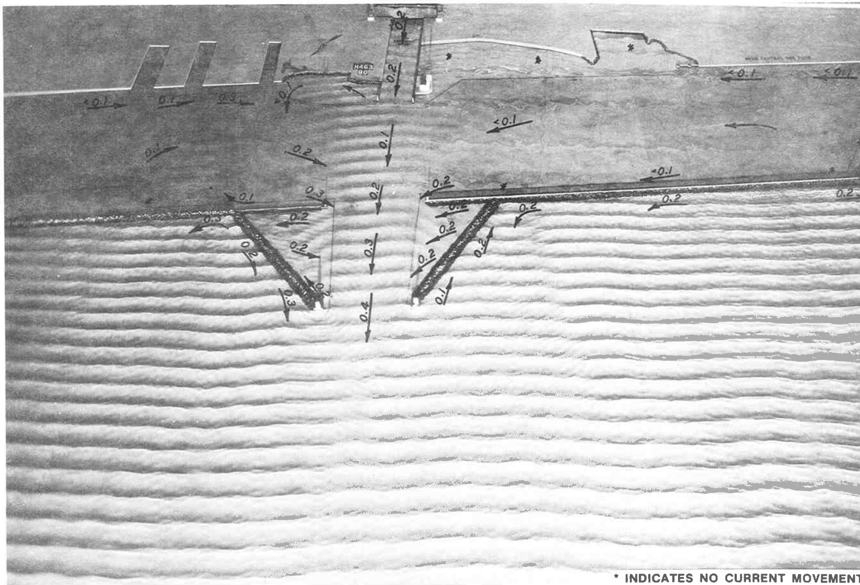
Photo 17. Typical wave patterns, current patterns, and current magnitudes (prototype feet per second) for existing conditions; 6-sec, 5.6-ft waves from 326 deg; +2.6 ft swl; river discharge 800 cfs
