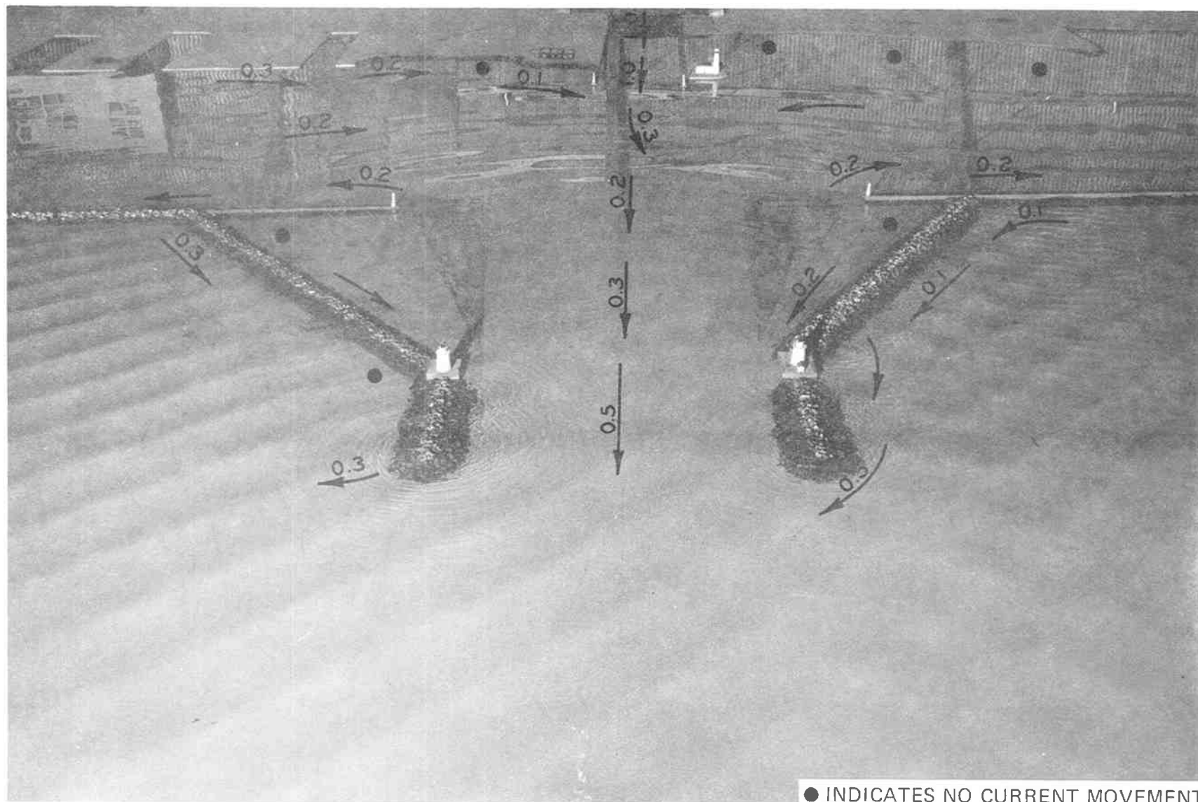
Photo 68. Typical wave patterns, current patterns, and current magnitudes (prototype feet per second) at the west entrance for Fair-Weather Plan 4D; 6-sec, 3.9-ft waves from 279 deg; +2.6 ft swl; river discharge 8,000 cfs
