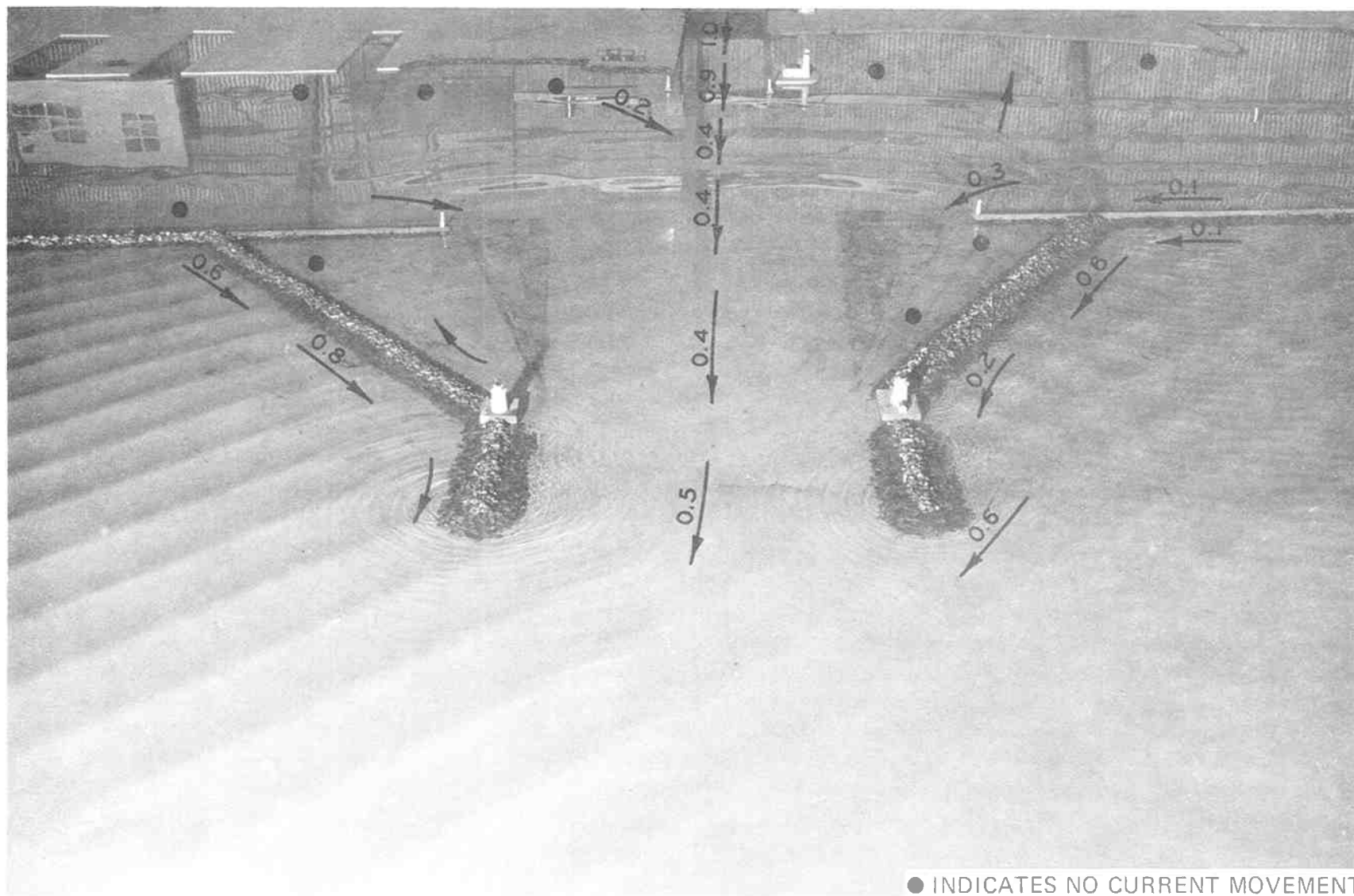
Photo 64. Typical wave patterns, current patterns, and current magnitudes (prototype feet per second) at the west entrance for Fair-Weather Plan 4D; 6-sec, 3.9-ft waves from 279 deg; 0.0-ft swl; river discharge 8,000 cfs
