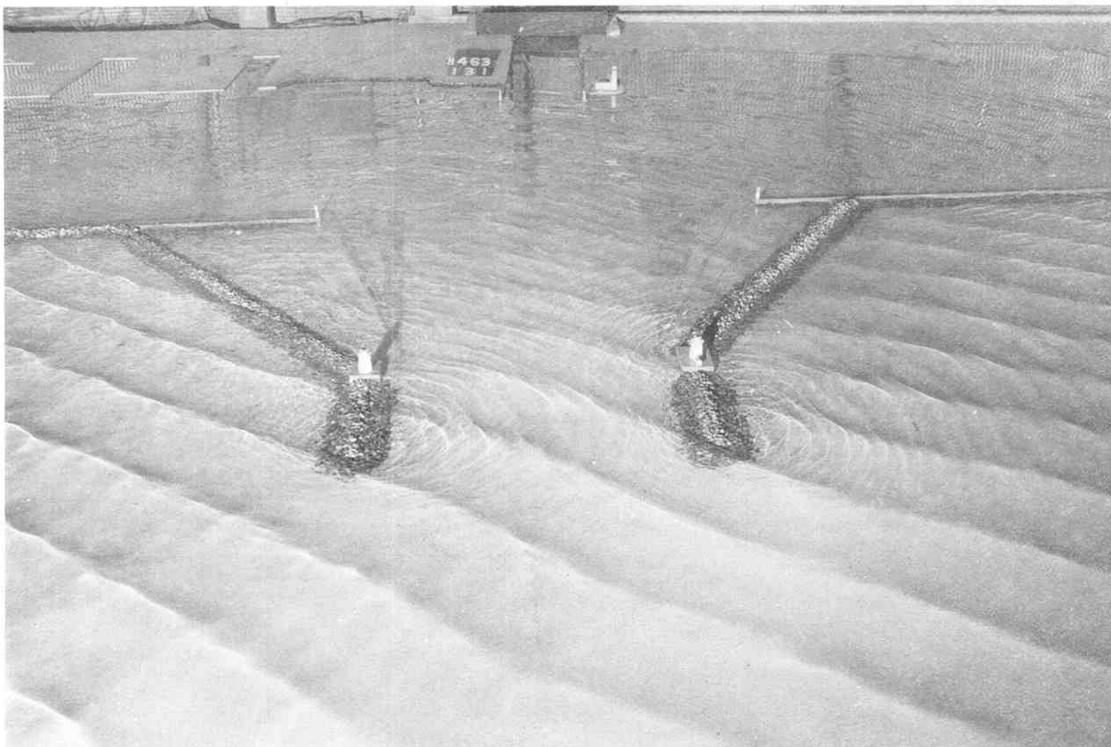
Photo 61. Typical wave patterns at the west entrance for Fair-Weather Plan 4D; 8-sec, 9.8-ft waves from 17 deg; +2.6 ft swl; river discharge 800 cfs
