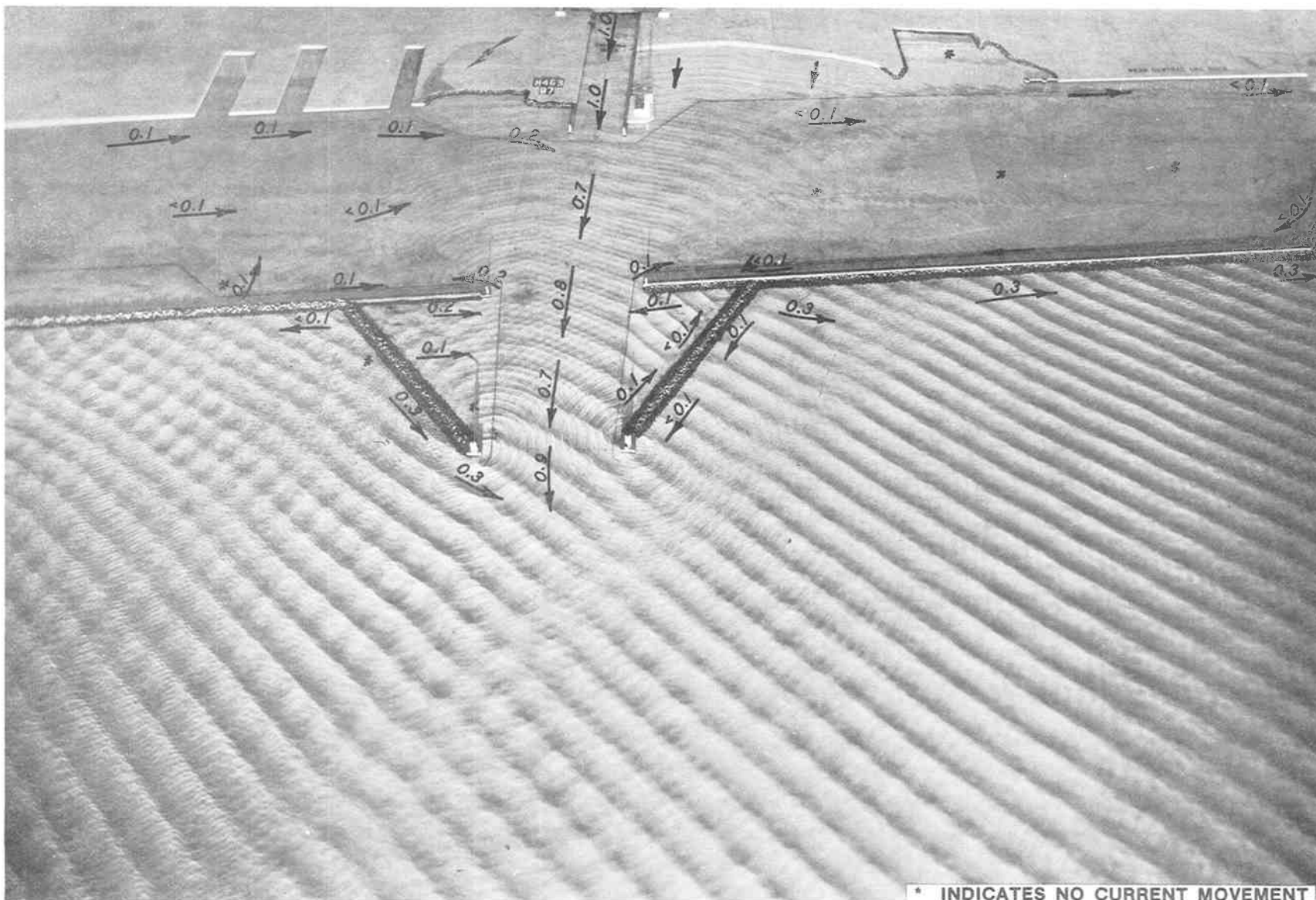
Photo 26. Typical wave patterns, current patterns, and current magnitudes (prototype feet per second) for existing conditions; 6-sec, 4.7-ft waves from 17 deg; 0.0-ft swl; river discharge 8,000 cfs
