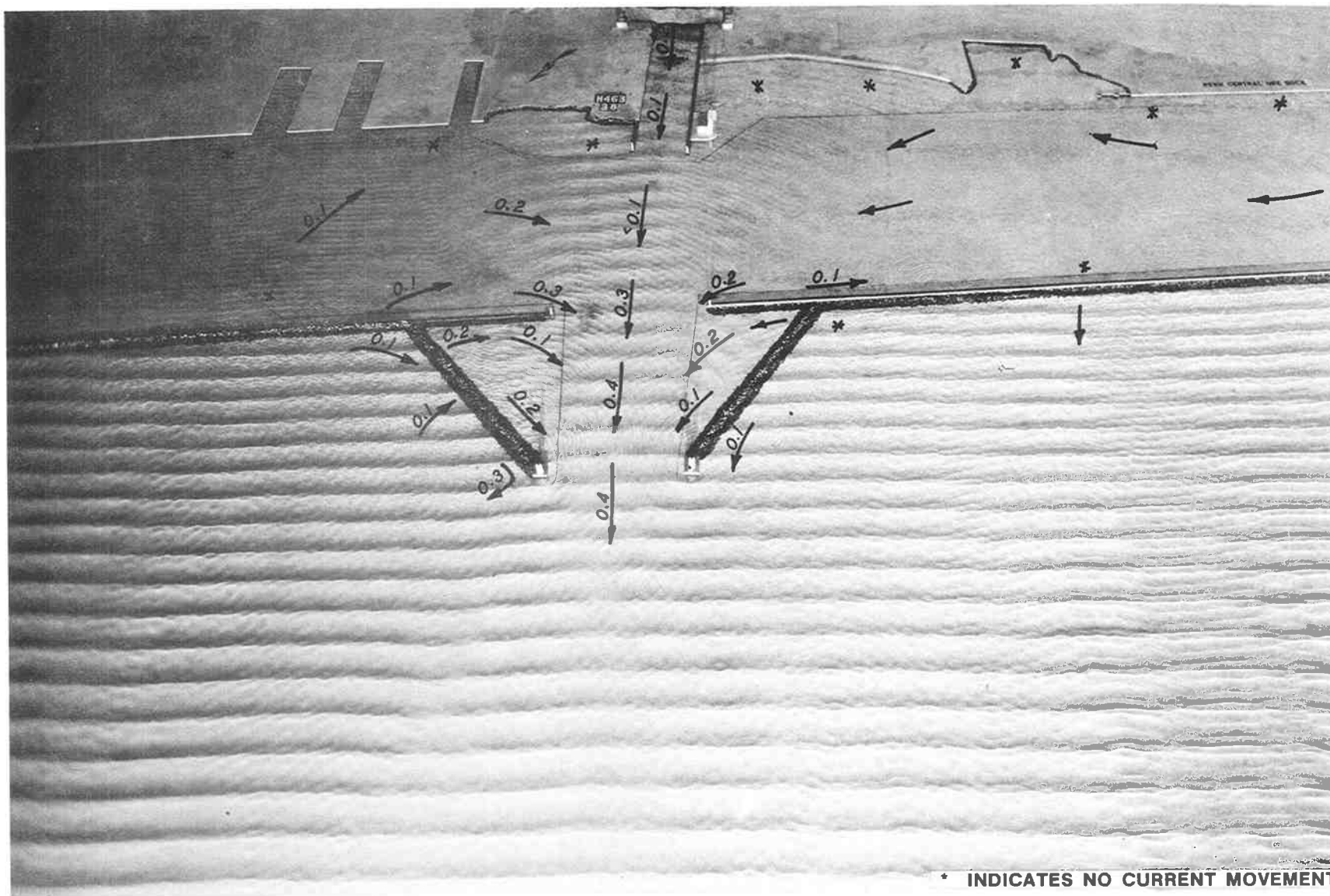
Photo 21. Typical wave patterns, current patterns, and current magnitudes (prototype feet per second) for existing conditions; 6-sec, 5.6-ft waves from 326 deg; +4.8 ft swl; river discharge 800 cfs
