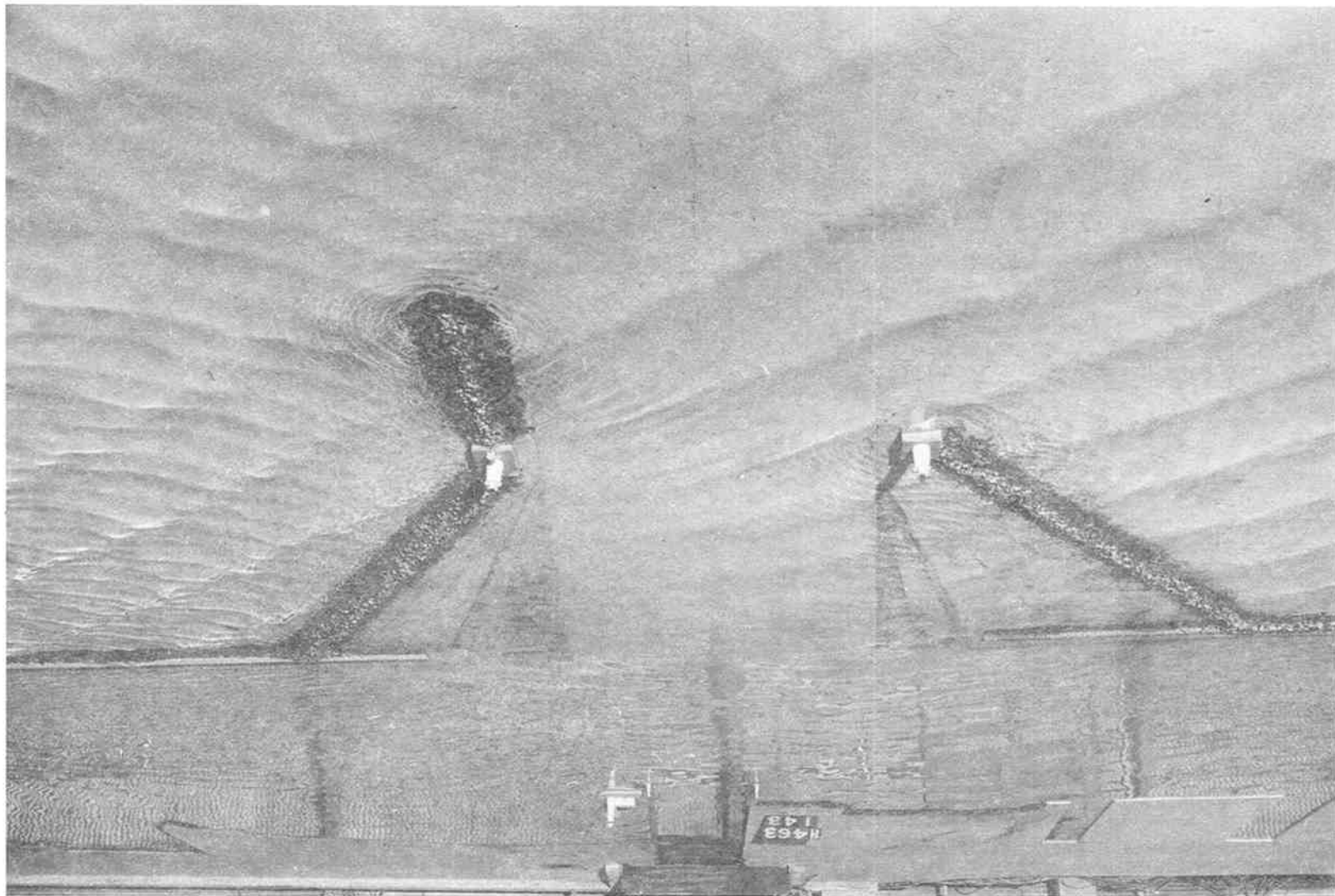
Photo 57. Typical wave patterns at the west entrance for Fair-Weather Plan 4; 9-sec, 8.6-ft waves from 279 deg; +2.6 ft SWL; river discharge 800 cfs
