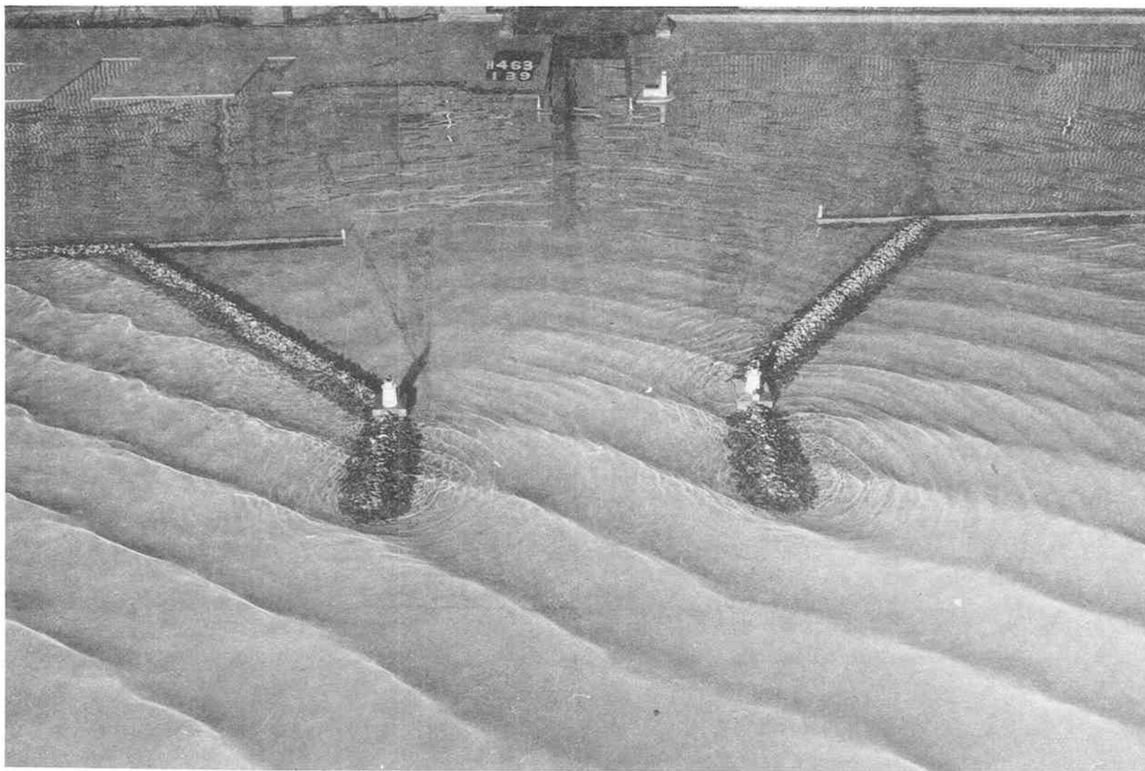
Photo 62. Typical wave patterns at the west entrance for Fair-Weather Plan 4E; 8-sec, 9.8-ft waves from 17 deg; +2.6 ft swl; river discharge 800 cfs
