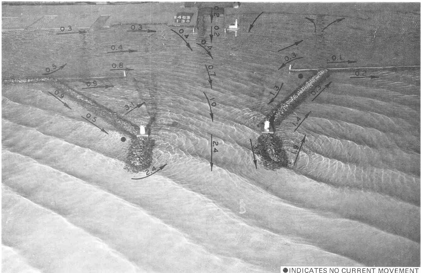
Photo 98. Typical wave patterns, current patterns, and current magnitudes (prototype feet per second) at the west entrance for Fair-Weather Plan 4D; 8-sec, 9.8-ft waves from 17 deg; +4.8 ft swl; river discharge 8,000 cfs
