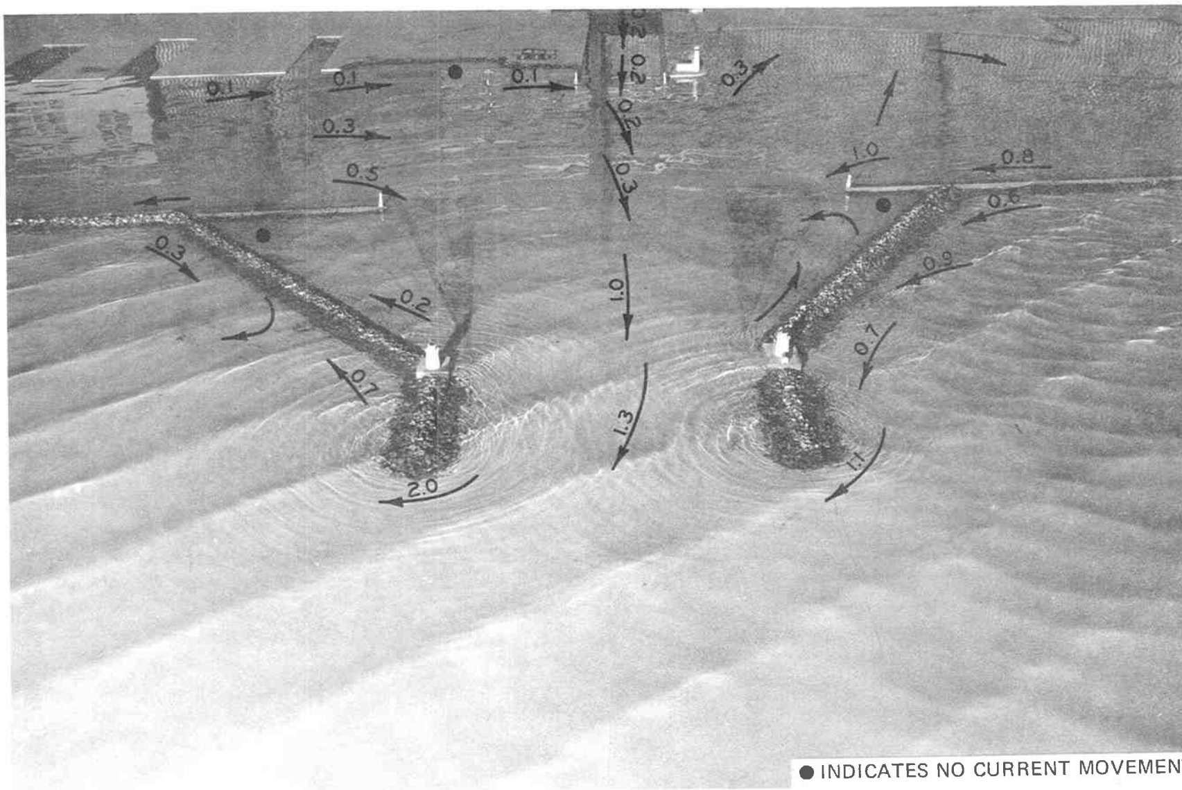
Photo 69. Typical wave patterns, current patterns, and current magnitudes (prototype feet per second) at the west entrance for Fair-Weather Plan 4D; 9-sec, 8.6-ft waves from 279 deg; +2.6 ft swl; river discharge 800 cfs
