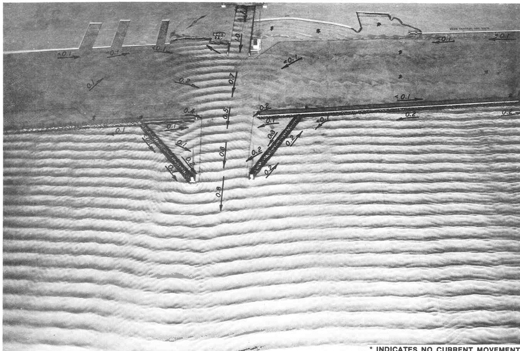
Photo 18. Typical wave patterns, current patterns, and current magnitudes (prototype feet per second) for existing conditions; 6-sec, 5.6-ft waves from 326 deg; +2.6 ft swl; river discharge 8,000 cfs
