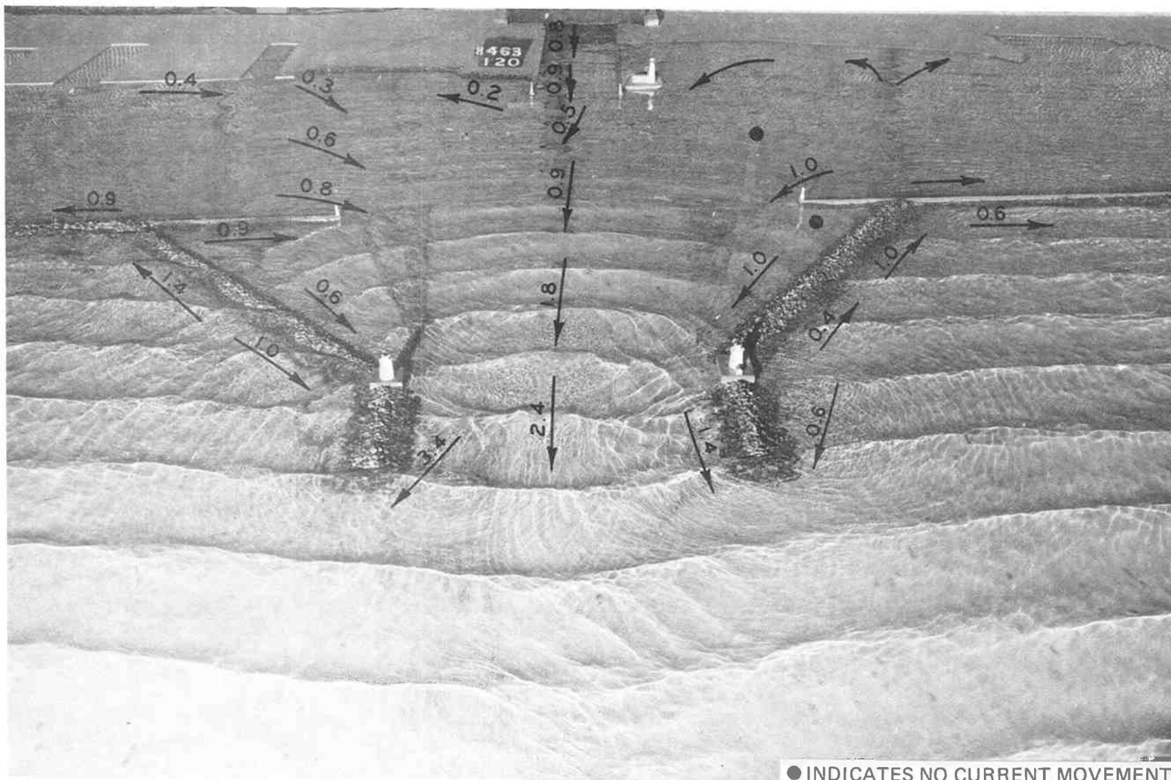
Photo 82. Typical wave patterns, current patterns, and current magnitudes (prototype feet per second) at the west entrance for Fair-Weather Plan 4D; 9-sec, 11.9-ft waves from 326 deg; +2.6 ft swl; river discharge 8,000 cfs
