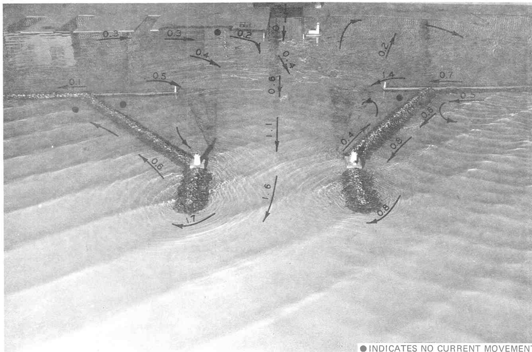
Photo 70. Typical wave patterns, current patterns, and current magnitudes (prototype feet per second) at the west entrance for Fair-Weather Plan 4D; 9-sec, 8.6-ft waves from 279 deg; +2.6 ft swl; river discharge 8,000 cfs
