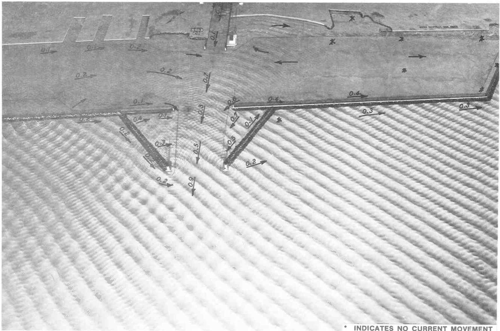
Photo 34. Typical wave patterns, current patterns, and current magnitudes (prototype feet per second) for existing conditions; 6-sec, 4.7-ft waves from 17 deg; +4.8 ft swl; river discharge 8,000 cfs
