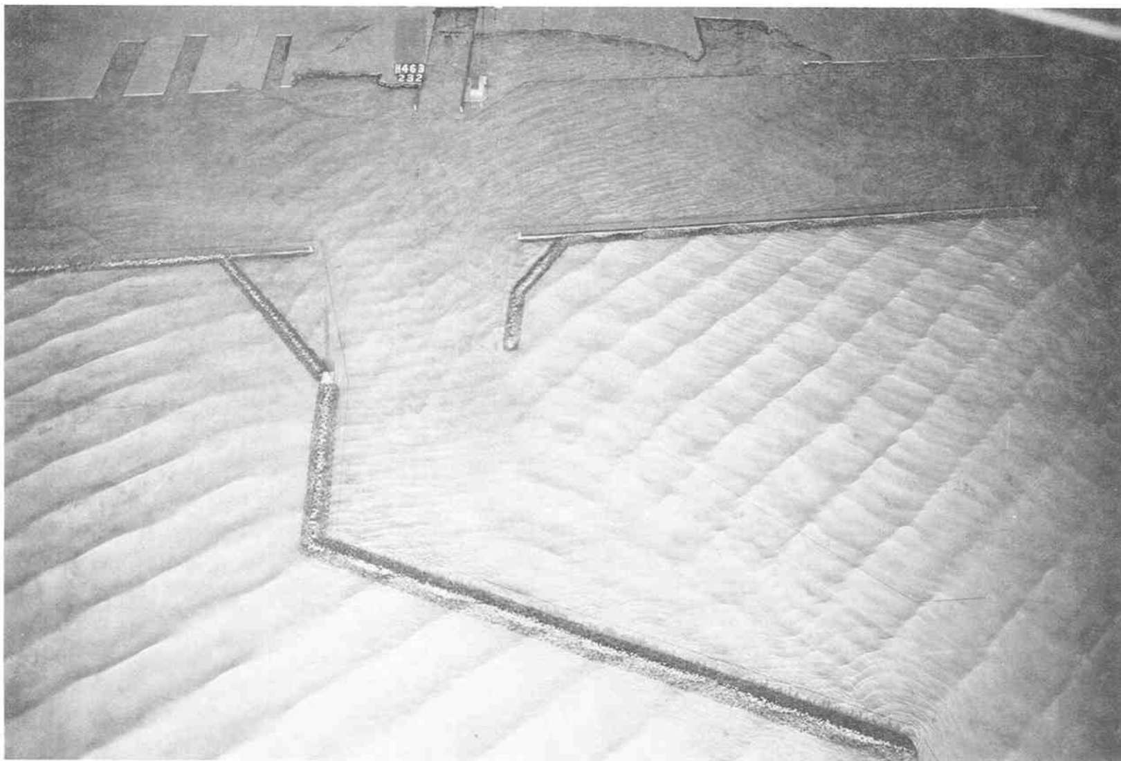
Photo 148. Typical wave patterns for Severe-Weather Plan 14; 10-sec, 9.2-ft waves from 279 deg; +4.8 ft swl; river discharge 800 cfs
