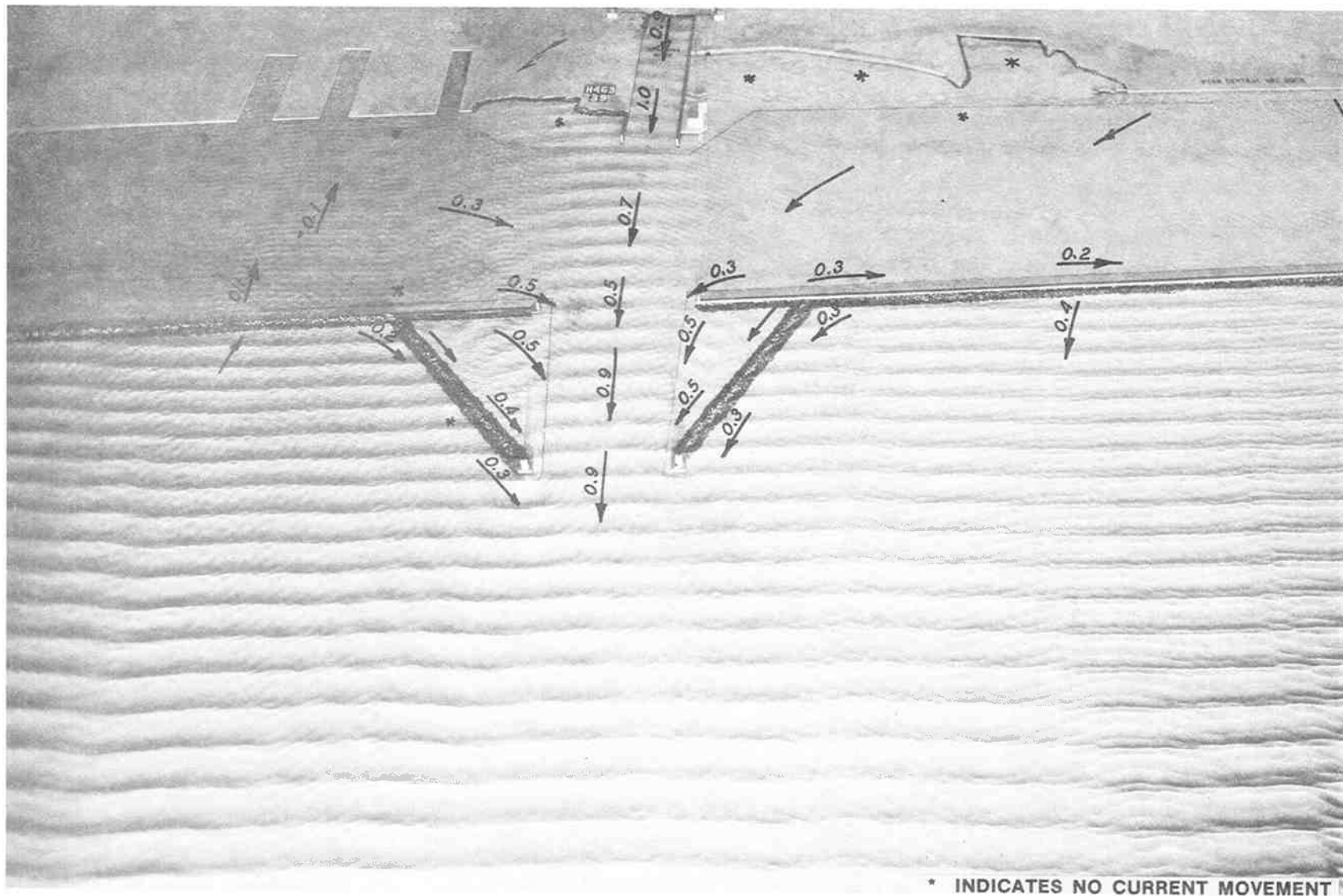
Photo 22. Typical wave patterns, current patterns, and current magnitudes (prototype feet per second) for existing conditions; 6-sec, 5.6-ft waves from 326 deg; +4.8 ft swl; river discharge 8,000 cfs
