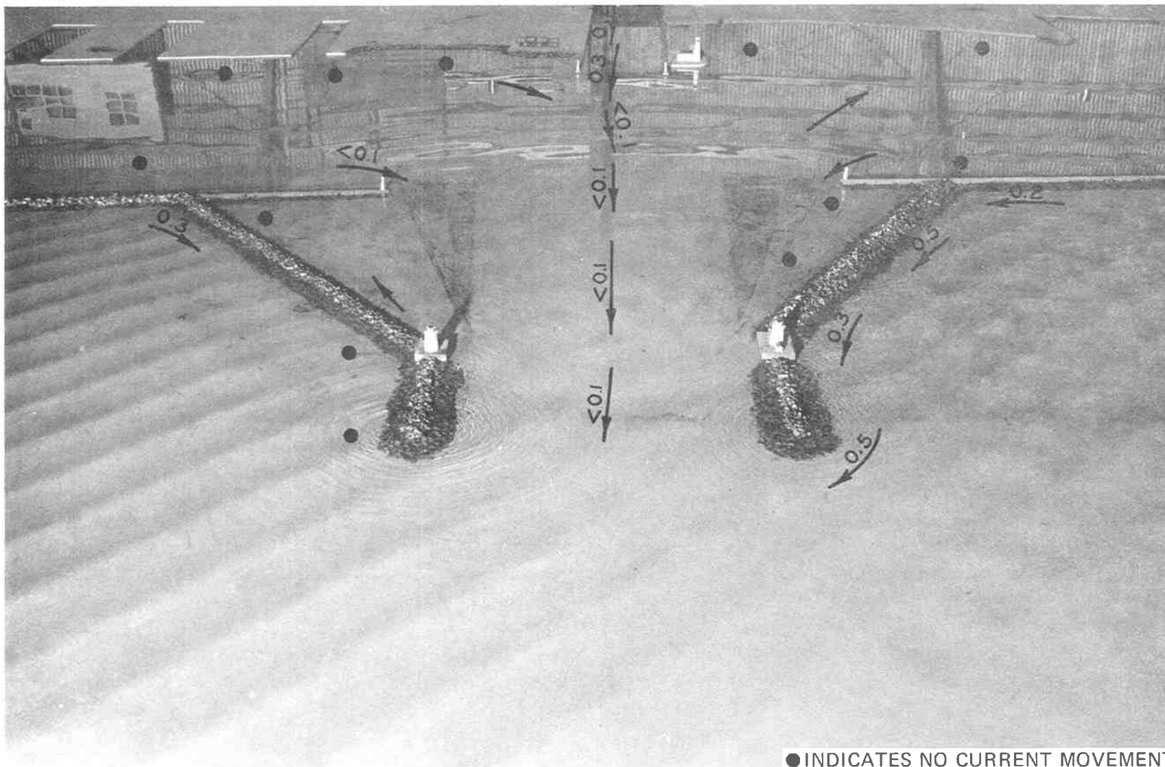
Photo 63. Typical wave patterns, current patterns, and current magnitudes (prototype feet per second) at the west entrance for Fair-Weather Plan 4D; 6-sec, 3.9-ft waves from 279 deg; 0.0-ft swl; river discharge 800 cfs
