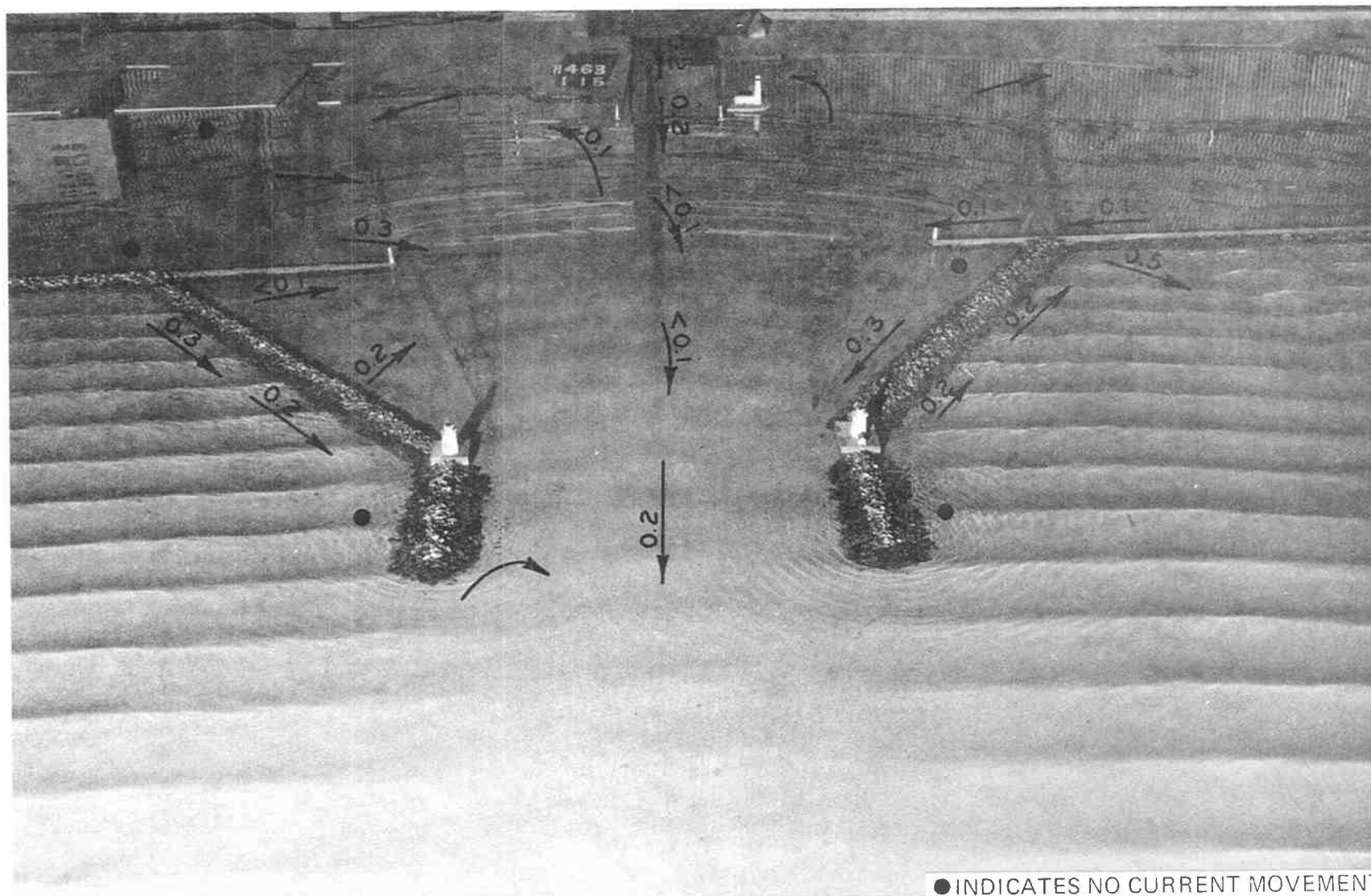
Photo 75. Typical wave patterns, current patterns, and current magnitudes (prototype feet per second) at the west entrance for Fair-Weather Plan 4D; 6-sec, 5.6-ft waves from 326 deg; 0.0-ft swl; river discharge 800 cfs
