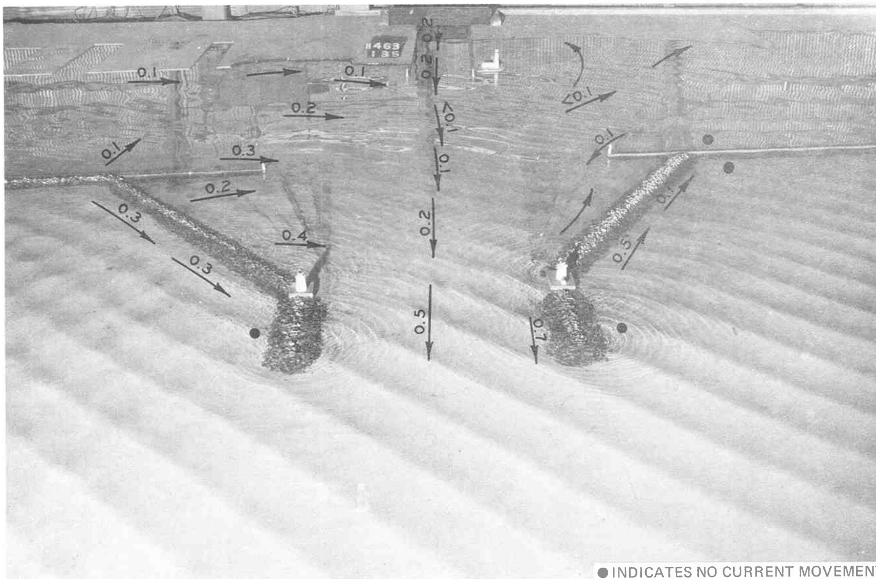
Photo 95. Typical wave patterns, current patterns, and current magnitudes (prototype feet per second) at the west entrance for Fair-Weather Plan 4D; 6-sec, 4.7-ft waves from 17 deg; +4.8 ft swl; river discharge 800 cfs
