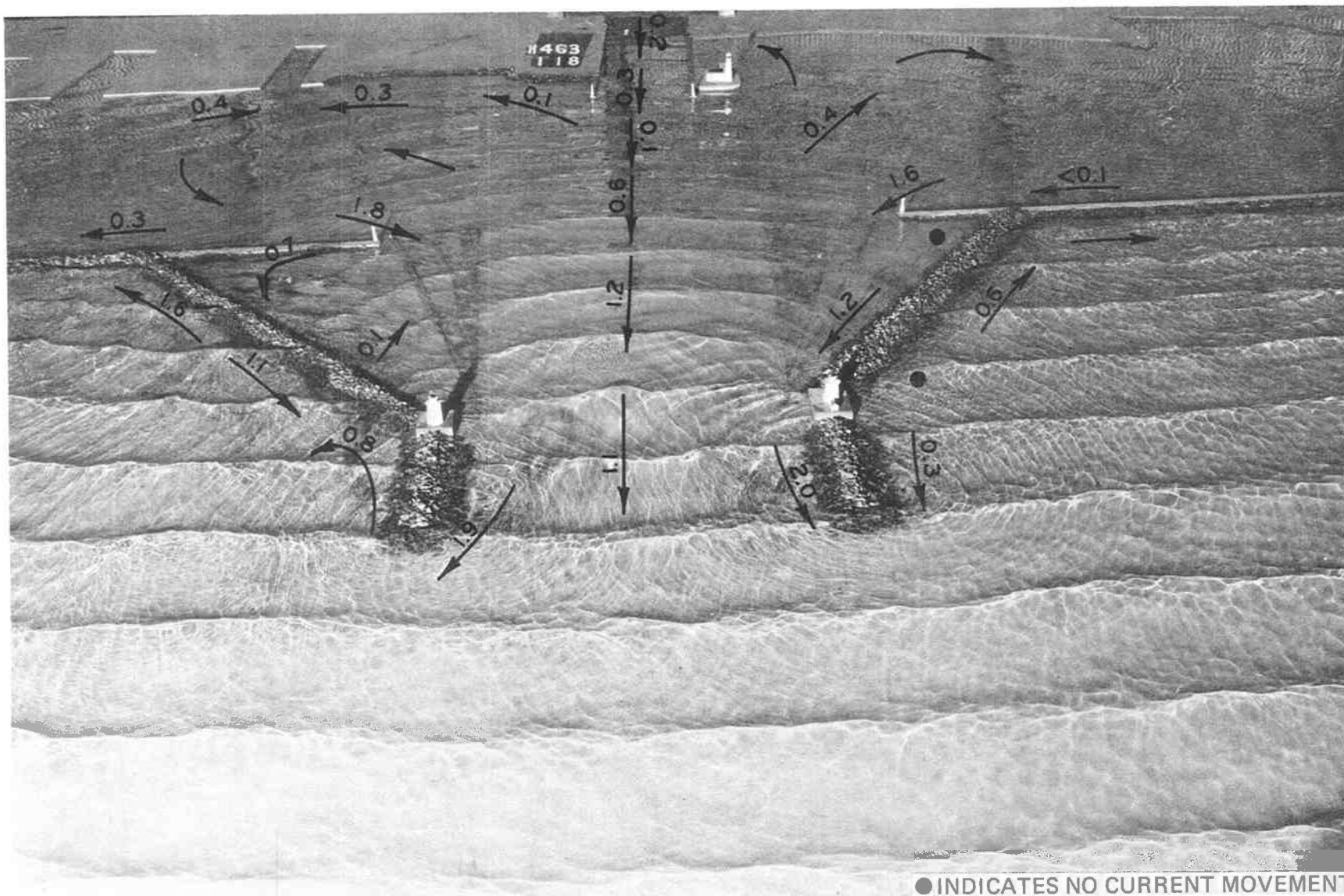
Photo 77. Typical wave patterns, current patterns, and current magnitudes (prototype feet per second) at the west entrance for Fair-Weather Plan 4D; 9-sec, 11.9-ft waves from 326 deg; 0.0-ft swl; river discharge 800 cfs
